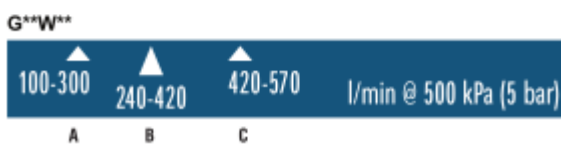
Figure 4.4B 1.5" / 38 mm G-Force 75 psi / 5 bar with flow limiting
