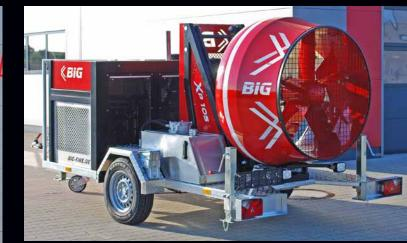
The logical integration of technology into the design of the trailer enables the XP 105 to be built as the first hydraulically driven MGV on an one-axle trailer and the integrated handles on the side allow fire fighters to position the MGV easily by hand. Despite the enormous lifting height, the MGV XP 105 only has a total height of less than 2 m in the transport position and can therefore be brought to the operation site even through low car passages.
