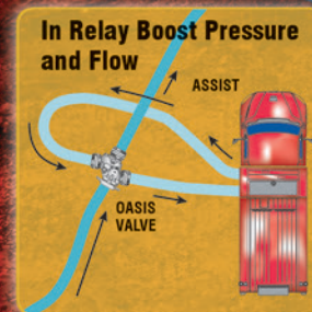
Boost pressure and flow with a hose lay of 500 feet plus.
