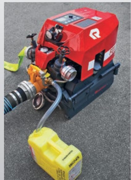
FOX with integrated foam proportioning system
