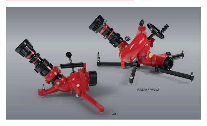
Portable monitors can be used for fire fighting, cooling or as a water shield. They can be used either manned or unmanned. Depending on the model and the tip used, throw ranges of up to 50 m (RB 6 with one inlet) or 55 m (POWER STREAM with two inlets) can be achieved.
